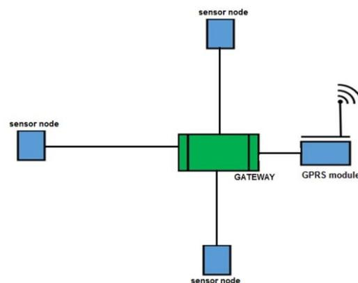
Figure 1: Schematic o of an Automatic Weather Station
