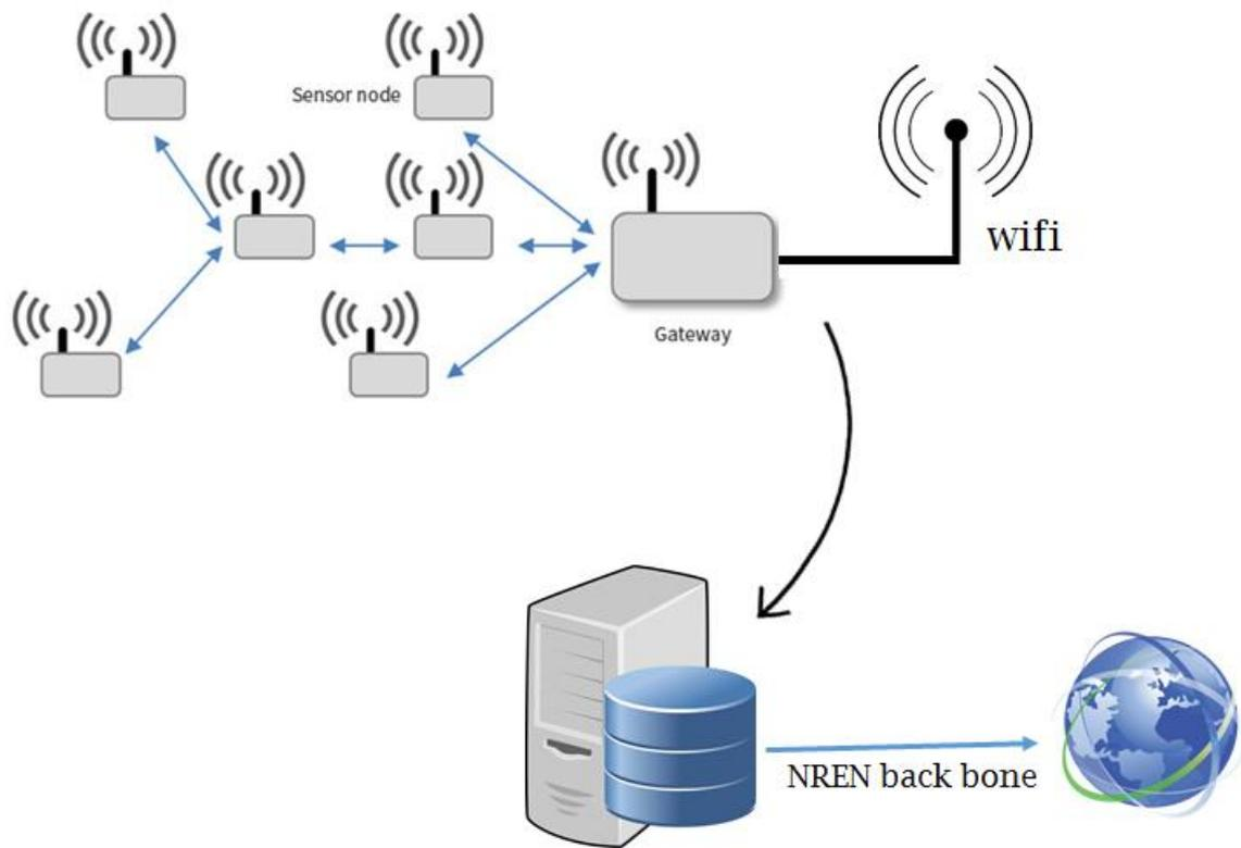
Figure 5: AWS network architecture
